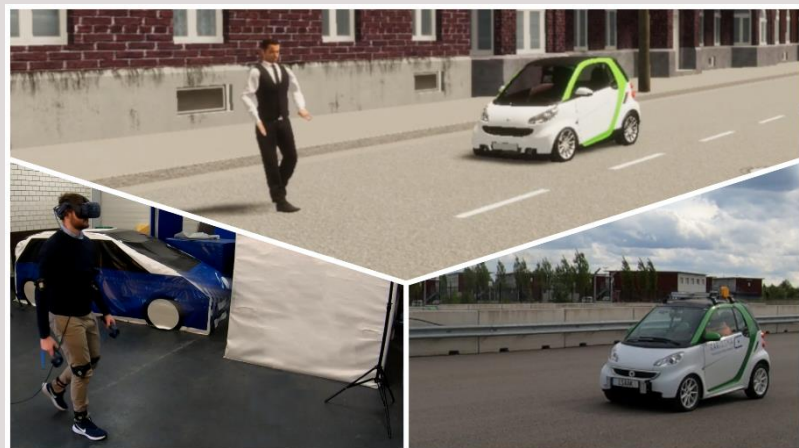
Fig. 3: The mixed reality test environment MiRe with the components simulation (top), pedestrian tracking (bottom left) and real vehicle (bottom right) Source THI
