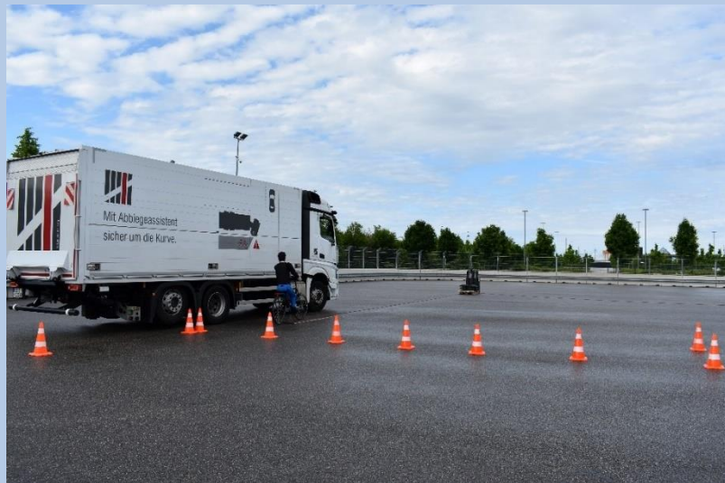
Fig. 4: Dynamic functional test of the Blind Spot Information System [own illustration] Source: THI
