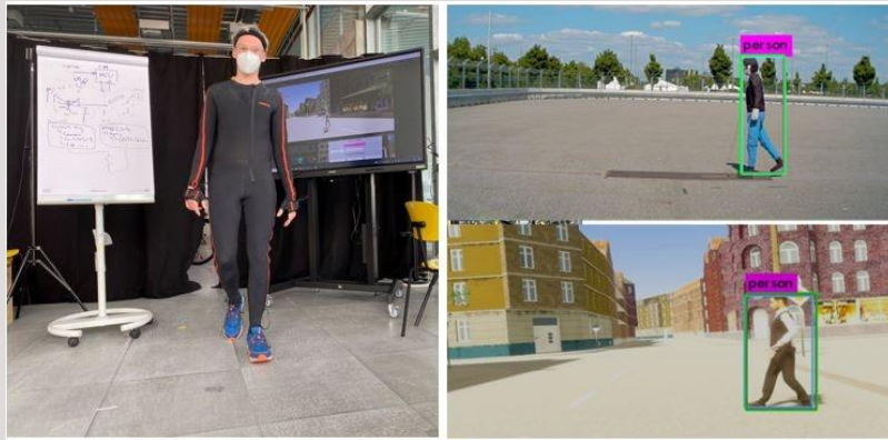
Fig. 2: Motion capturing system (left), real pedestrian dummy with object recognition (top right) and pedestrian model in the simulation (bottom right) Source: THI
