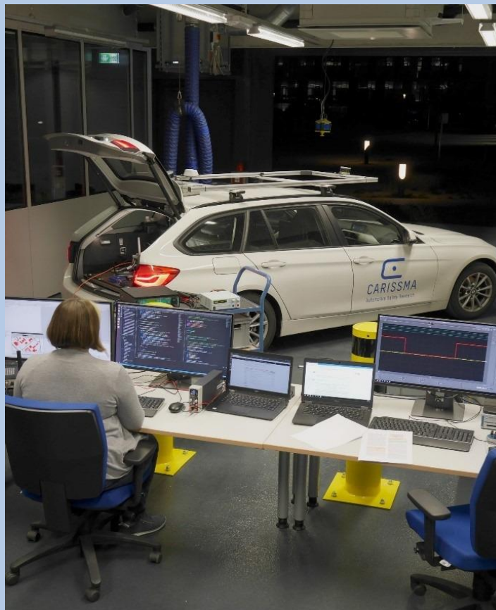
Fig. 4: Test setup Coupling Car2X simulation with test vehicle for reliability evaluation. (Source: THI)
