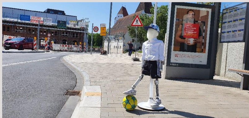
Fig. 3: Dummy with movable joints and artificial muscles. (Source: THI)
