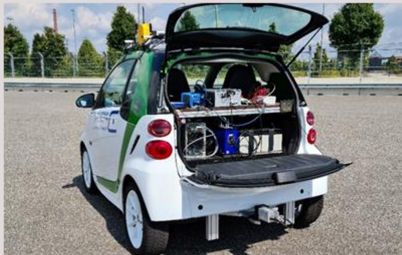
Fig. 1: Shown is a test vehicle that is equipped with an ADMA G-Pro+, a Correvit S-Motion and a car pc. (Source: THI)
