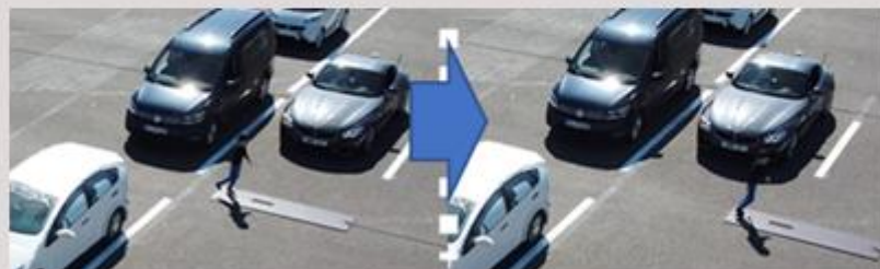
Fig. 5: Shown is the recreation of a real-life traffic scenario on the outdoor test facility. A pedestrian attempts to cross a street, and a vehicle performs an emergency braking to avoid a collision. (Source: THI)
