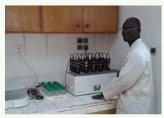
Automatic Methane Potential Test System to assess the biochemical methane potential of bio-wastes, located at the ISRA/IRD research centre of Dakar, Senegal (September 2015). © J.-M. Médoc
