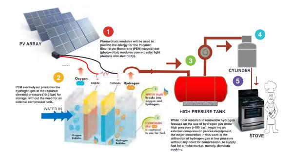
Design of PV array to power electrolyser
