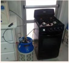
Modified stove with specialised  $H_2$  gas burners connected to a low pressure gas storage cylinder and PEM electrolyser powered by a PV system (June 2015).
