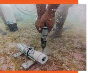
Deploying a pressure sensor on Fatato reef, Funafuti, Tuvalu. The data is analysed to extract short wave and infragravity wave information in order to gain insight on wave transformation on reef-fronted islands (April 2013).
